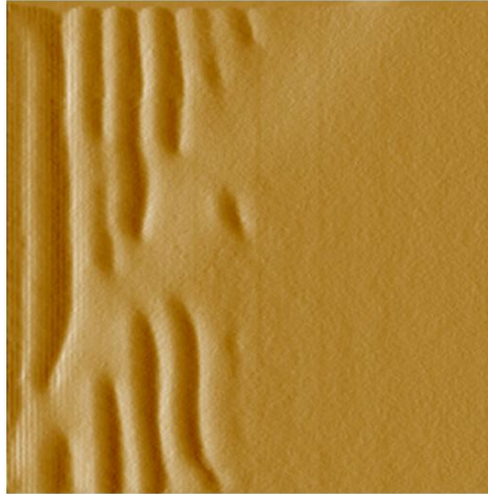
Figure 2.20. A 300 nm tilt over 12 \mu\text{m} showing the ripple patten propagation at the bottom slope of the sample.
