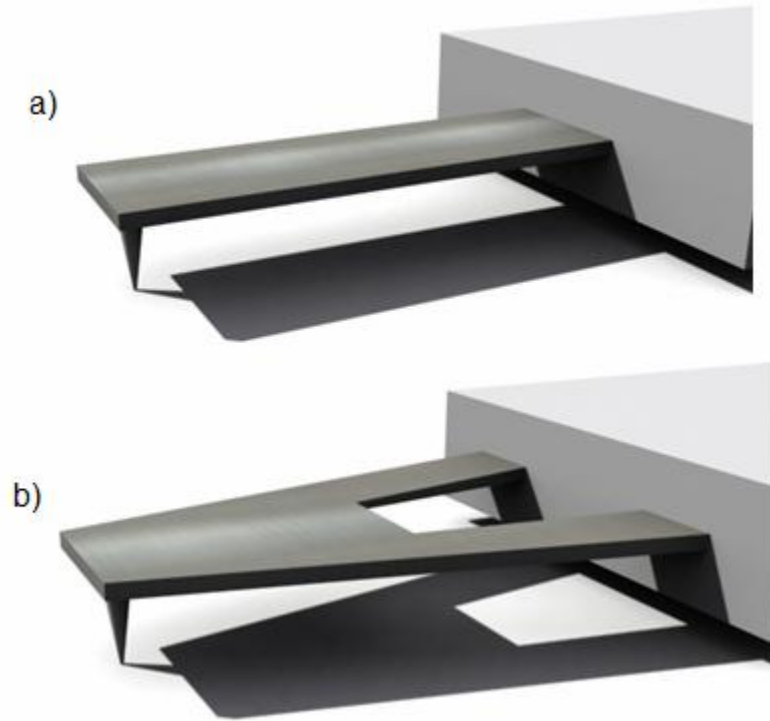
Figure 3.1. Schematic of a) tapping mode tip and b) contact mode tip (dual cantilever).
